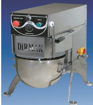
**IBT 12-VE** 10 l planetary mixer, stainless steel safety cover, with electronic speed variation (21 –201 rpm). Oil-less planetary system. Tabletop usage. Equipped with spiral hook, paddle, whisk 10 l stainless steel bowl.
