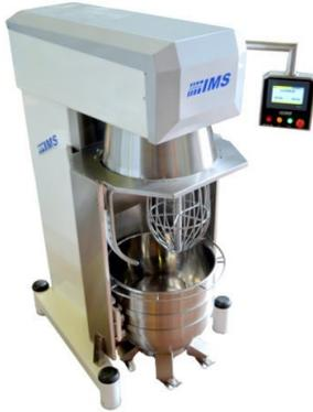
**IBT 140-VEL** 140 l planetary mixer, stainless steel safety cover, with electronic speed variator (20 –215 rpm). Lifting system for Up/Down bowl. Oil-less planetary system. 7" Touchscreen panel for controlling machine. Equipped with spiral hook, paddle, whisk. Bowl with wheels.
