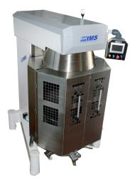
IBT 200-VEL 200 I planetary mixer, stainless steel safety cover, with electronic speed variator (20 –245 rpm). Lifting system for Up/Down bowl. Oil-less planetary system. 10" Touchscreen panel for machine control. Leakproof cover for bowl. Safety cover for bowl movement. Equipped with spiral hook, paddle, whisk and scraper. Bowl with wheels.
