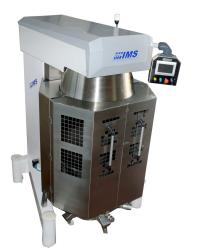
IBT 300-VEL 300 l planetary mixer, stainless steel safety cover, with electronic speed variator (20 –245 rpm). Lifting system for Up/Down bowl. Oil-less planetary system. 10" Touchscreen panel for machine control. Leakproof cover for bowl. Safety cover for bowl movement. Equipped with spiral hook, paddle, whisk and scraper. Bowl with wheels.
