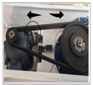
Check the belt tension and degree of wear. To check it, proceed as follows:
