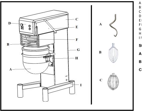
A Stainless steel bowl B Safety guard C Head D Control panel E Lift/lower lever F Planetary gear system G Column H Bowl cradle I Feet
